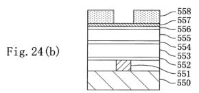
Figure 24(b), reproduced above, is a cross-sectional view of a partially formed interconnection structure during a process step for forming the same. *Id.* at 9:28–31. In this step, first resist pattern 558 is formed on titanium nitride film 557. *Id.* at 25:19–21. First resist pattern 558 includes openings for forming wiring grooves of the interconnection structure. *Id.*
