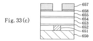
Figure 33(c), reproduced above, is a cross-sectional view of a partially-formed interconnection structure during a process step for forming the same. Ex. 1001, 9:60–63. In this step, titanium nitride film 656 is dry-etched using first resist pattern 657 as a mask, thereby forming mask pattern 658. *Id.* at 30:38–40.
