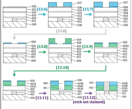
Transfer wiring pattern Transfer via pattern Transfer wiring pattern and via pattern
