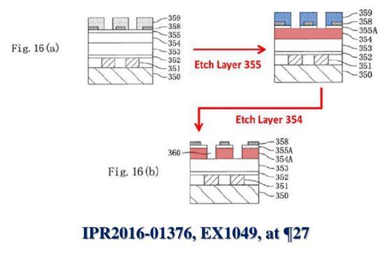
second silicon dioxide film 355. Then, the second silicon dioxide film 355 and the organic film 354 are sequentially dry-etched using the second resist pattern 359 as a mask, thereby forming a patterned second silicon dioxide film 355A and a patterned organic film 354A having openings 360 for forming contact holes as shown in FIG. 16(b). In this case, the second resist pattern 359 is removed during the step of etching the organic film 354.
