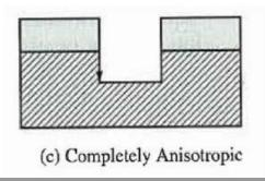
chemical etching and anisotropic physical etching as illustrated in Figure 10-3(b). Instead, the profile for ion-enhanced etching is much more like the case for physical etching acting alone, as in Figure 10-3(c). If the chemical component in the etch system is increased, the vertical etching is increased but not the lateral etching, which is not what would be expected from chemical etching....
