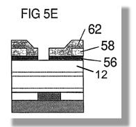
transferring, at least partially concurrently, said via pattern into said first dielectric layer to form via cavities corresponding to said via pattern, and said wiring pattern into said second dielectric layer to form wiring cavities corresponding to said wiring pattern, and
