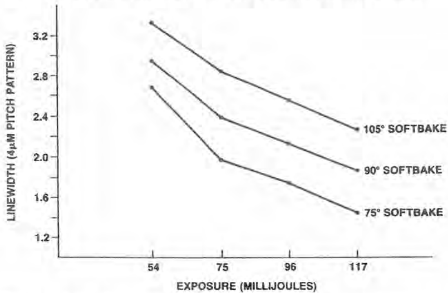
Figure 34. Critical dimension vs. exposure for OFPR-800 photoresist process.
