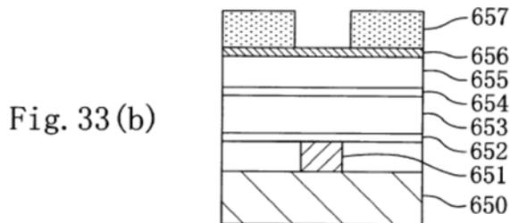
Figure 33(b), reproduced above, is a cross-sectional view of a partially-formed interconnection structure during a process step for forming the same. *Id.* at 9:60–63. In this step, first resist pattern 657 is formed on titanium nitride film 656. *Id.* at 30:36–37. First resist pattern 657 includes openings for forming wiring grooves of the interconnection structure. *Id.*
