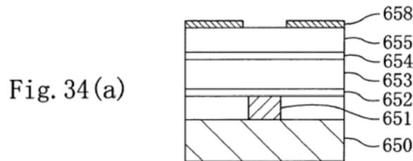
Figure 34(a), reproduced above, is a cross-sectional view of a partially-formed interconnection structure during a process step for forming the same. *Id.* at 9:64–67. In this step, first resist pattern 657 is removed. *Id.* at 30:44–45.
