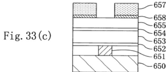
Figure 33(c), reproduced above, is a cross-sectional view of a partially-formed interconnection structure during a process step for forming the same. Ex. 1001, 9:60–63. In this step, titanium nitride film 656 is dry-etched using first resist pattern 657 as a mask, thereby forming mask pattern 658. *Id.* at 30:38–40.
