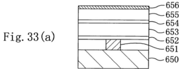
Figure 33(a), reproduced above, is a cross-sectional view of a partially-formed interconnection structure during a process step for forming the same. Ex. 1001, 9:60–63. As seen in Figure 33(a), silicon nitride film 652 is formed over first metal interconnects 651, which are formed on semiconductor substrate 650. *Id.* at 30:1–3. First organic film 653, silicon dioxide film 654, second organic film 655, and titanium nitride film 656 are deposited sequentially. *Id.* at 30:6–16.
