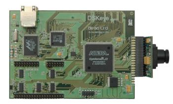
The DSKeye from BiTEC Ltd is a TI DSK daughterboard gathering the latest FPGA technology, a 5.2 mega pixel camera and user configurable interface options to deliver a Smart Camera system for development and research at a fraction of the cost normally associated with such technology.
