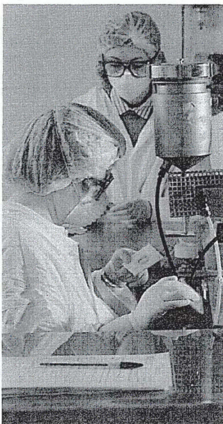
Fig. 10.5 Pilot scale manufacture of transdermal patches. (Courtesy of Elan Corporation, plc.)
