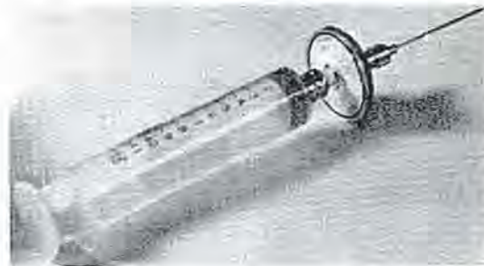
Fig. 14.6 Luer-Lock syringe adapted with a MILLEX Filter Unit and hypodermic needle. (Courtesy of Millipore Corporation.)
