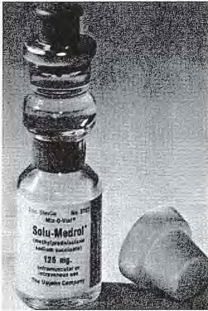
Fig. 14.10 The Mix-O-Vial shown above is a combination vial containing dry ingredients in the bottom compartment and a liquid diluent in the top compartment, separated by a specially formulated center seal. The bottom compartment can either be liquid filled, frozen and dried to make a lyophilized product, or it may be powder filled. The top diluent contains a preservative and may or may not contain one or more active ingredients. To use the vial, the dust cover is removed (as shown above), pressure is applied with the thumb to the top plunger which dislodges the center seal and the vial is shaken until the solution is effected. The top of the plunger is then swabbed with a disinfectant; the syringe needle inserted through the target circle on the plunger and the contents of the vial withdrawn into the syringe. The Mix-O-Vial offers stability of product (until it is activated), convenience, fast operation and safety as regards the right drug with the proper diluent in the correct proportions. (Courtesy of The Upjohn Company.)
