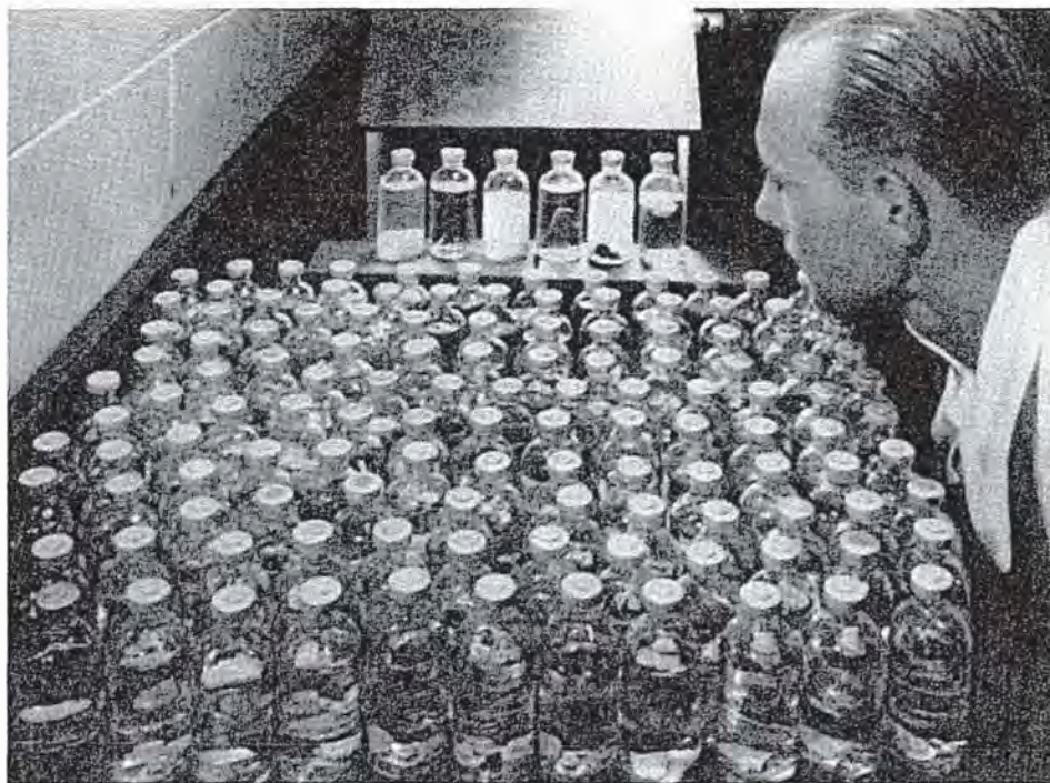
Fig. 14.14 Testing compatibility of rubber closures with the solution with which they are in contact. (Courtesy of Abbott Laboratories.)
