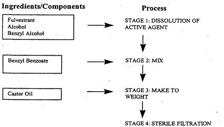
STAGE 4: STERILE FILTRATION (0.2µm) INTO BULK RECEIVING VESSEL
