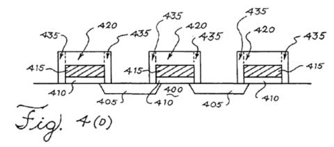
Figure 4(D) illustrates a cross-sectional view of a series of gates 415 (also called conducting layers or polysilicon layers) completely encapsulated in insulating material 420, e.g., TEOS (tetraethyl orthosilicate glass), where spacers or spacer portions 435 of the insulating material adjacent to the gates
