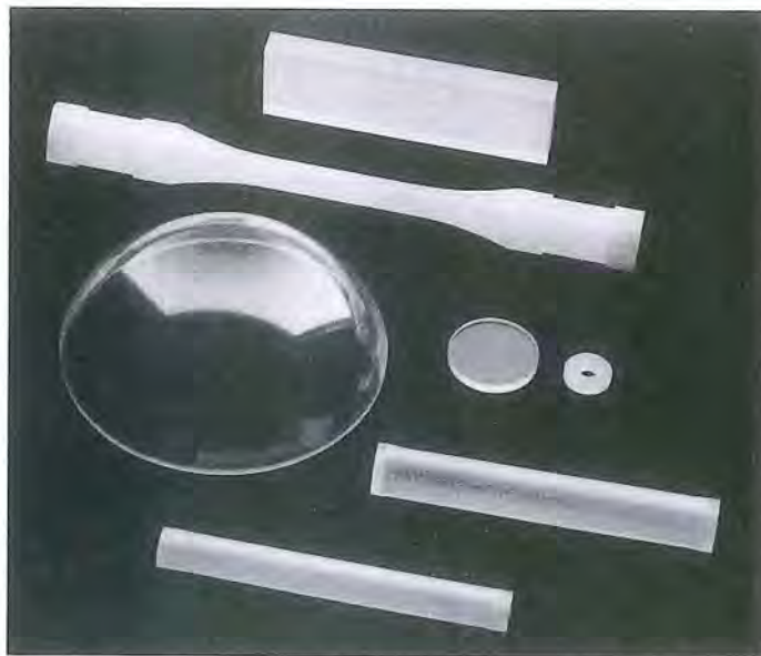
FIGURE 8-36 Pore-free sintered ceramic products. Tubes in the foreground are used in sodium vapor lamps and are made of translucent \text{Al}_2\text{O}_3 . The clear dome, tensile bar, and other shapes are composed of \text{Y}_2\text{O}_3 strengthened with \text{La}_2\text{O}_3 . Courtesy of W. H. Rhodes, Osram Sylvania.
