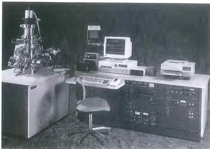
FIGURE 2-8 Photograph of an Auger electron spectrometer. Courtesy of Perkin-Elmer Physical Electronics Division.
