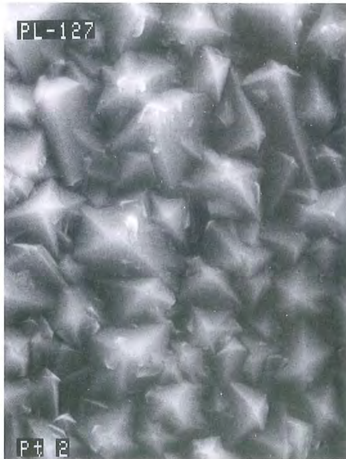
FIGURE 5-8 Diamond crystals grown by low-pressure CVD methods. Courtesy of T. R. Anthony, GE Corporate Research and Development.
