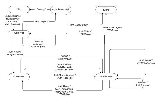
Figure 131—Authorization state machine flow diagram
