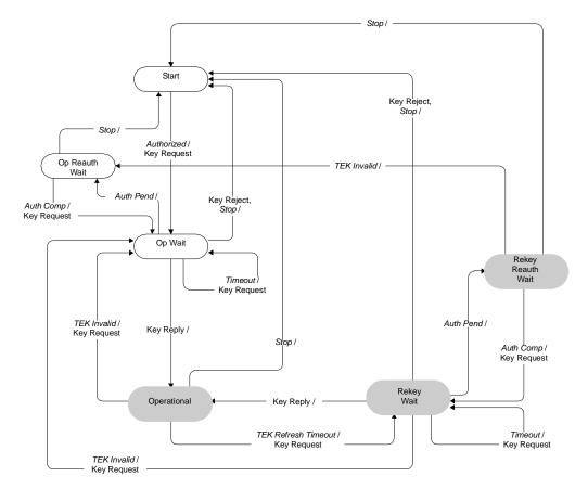
Figure 132—TEK state machine flow diagram
