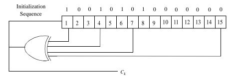
Figure 243—PRBS for ranging code generation
