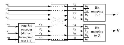
Figure 167—Optional pragmatic TCM encoder for rate 7/8 256-QAM
