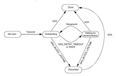
Figure 33—ARQ transmit block states
