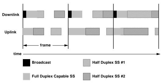
Figure 138—Example of FDD bandwidth allocation
