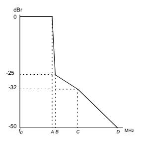
Figure 265—Transmit spectral mask (see Table 341)
