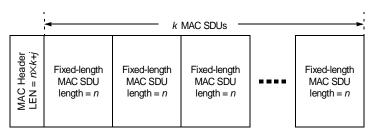
Figure 26—Packing fixed-length MAC SDUs into a single MAC PDU
