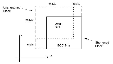
Figure 156—Structure of shortened 2 D block
