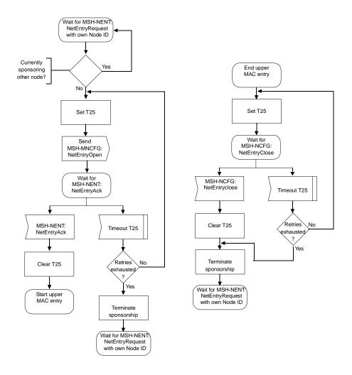
Figure 75—Mesh network synchronization and entry—Sponsor node
