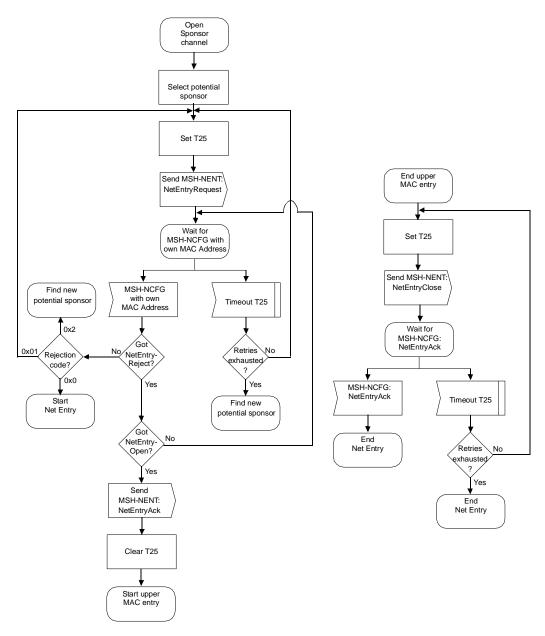
Figure 74—Mesh network synchronization and entry—New node—II
