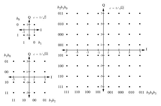
Figure 263—QPSK, 16-QAM, and 64-QAM constellations
