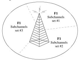
Figure B.6—Reuse of 1 configuration, 3 sectors per cell
