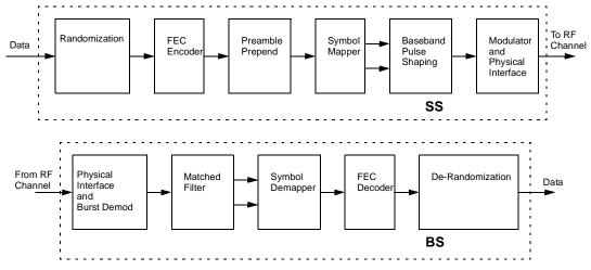
Figure 155—Conceptual block diagram of the uplink PHY
