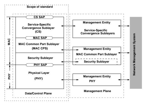
Figure 1—IEEE Std 802.16 protocol layering, showing SAPs
