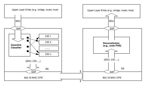
Figure 7—Classification and CID mapping (BS to SS)
