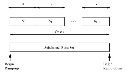
Figure 190—Forming of subchannel burst set from segments
