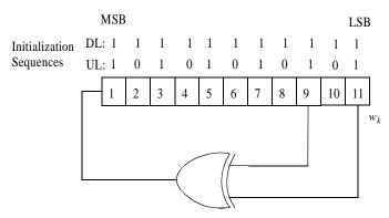
Figure 204—PRBS for pilot modulation
