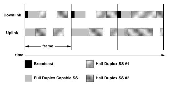
Figure 44—Example of Burst FDD bandwidth allocation
