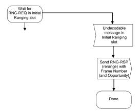
Figure 64—Initial ranging—BS response to undecodable message
