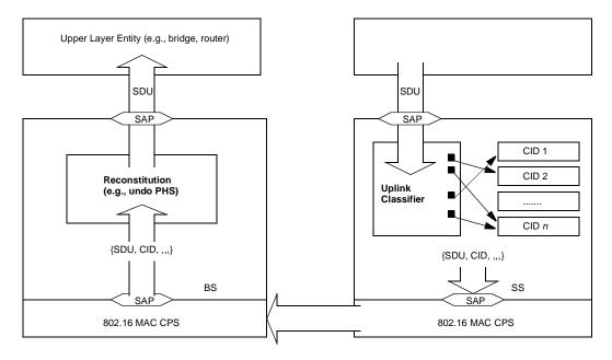
Figure 8—Classification and CID mapping (SS to BS)
