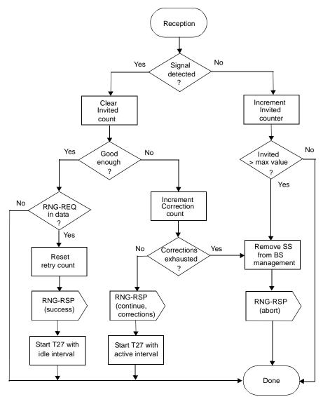
Figure 82—Periodic Ranging receiver processing—BS
