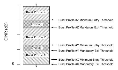
Figure 81—Burst profile threshold usage
