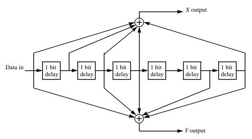
Figure 161—Binary rate 1/2 convolutional encoder
