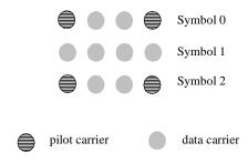
Figure 236—Description of an uplink tile
