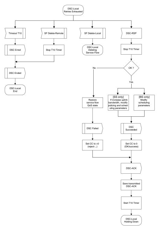
Figure 118—DSC—Locally Initiated Transaction Retries Exhausted state flow diagram
