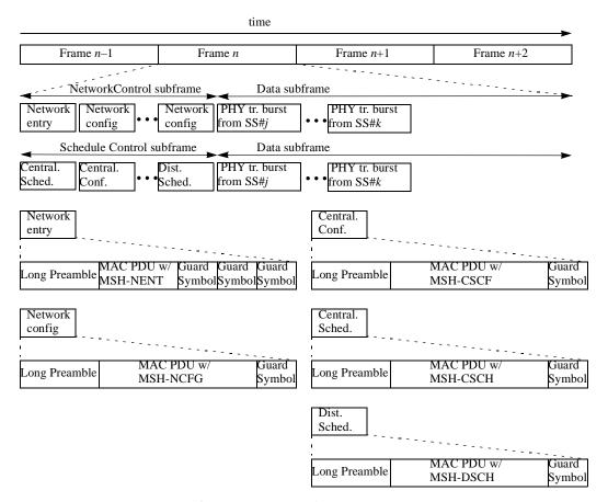
Figure 210—Mesh frame structure
