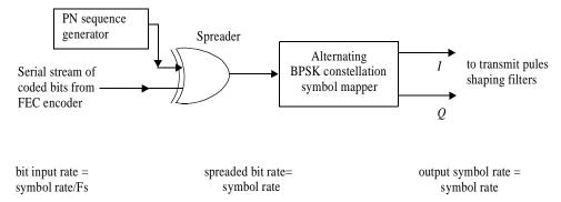
Figure 176—Spread BPSK processing
