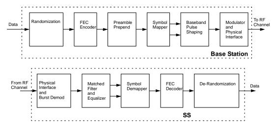
Figure 145—Conceptual block diagram of the downlink PMD sublayer
