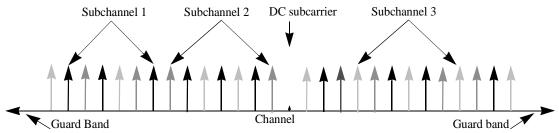
Figure 214—OFDMA frequency description (3 channel schematic example)
