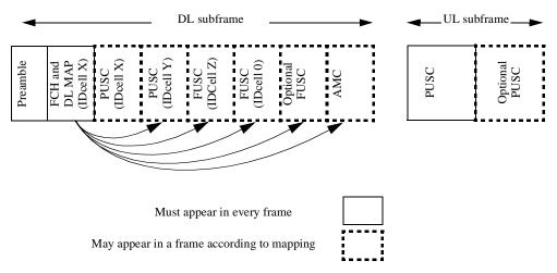
Figure 219—Illustration of OFDMA frame with multiple zones
