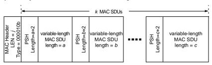
Figure 27—Packing variable-length MAC SDUs into a single MAC PDU
