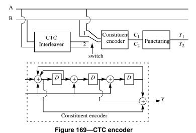
First, the encoder (after initialization by the circulation state  $Sc_1$ , see 8.2.1.2.4.2) is fed the sequence in the natural order (position 1) with the incremental address i = 0,...,N-1. This first encoding is called  $C_1$  encoding. Then the encoder (after initialization by the circulation state  $Sc_2$ , see in subclause 8.2.1.2.4.2) is fed by the interleaved sequence (switch in position 2) with incremental address j = 0,...,N-1. This second encoding is called  $C_2$  encoding.
