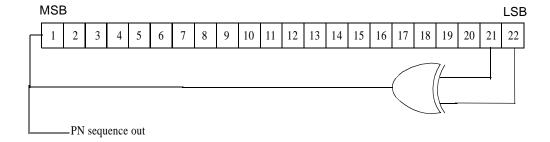
Figure 177—Spreading PN sequence generator
