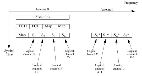
Figure 248— Example of using FHDC in PUSC
