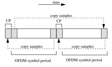
Figure 239—Initial-ranging transmission for OFDMA
