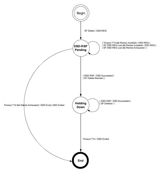
Figure 104—DSD—Locally Initiated Transaction state transition diagram
