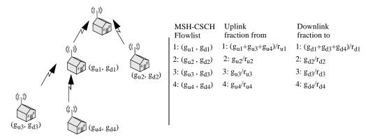
Figure 42—MSH-CSCH flow usage example
