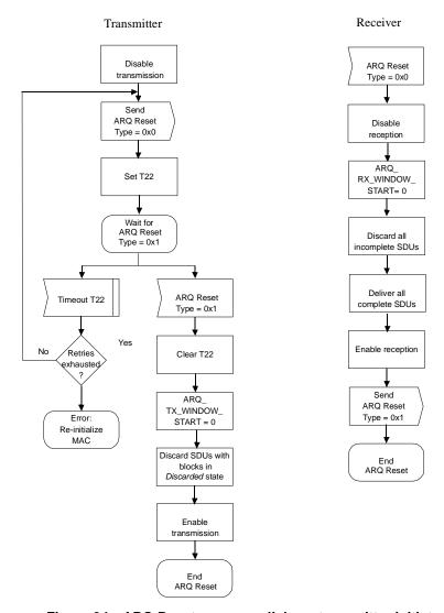
Figure 34—ARQ Reset message dialog—transmitter initiated
