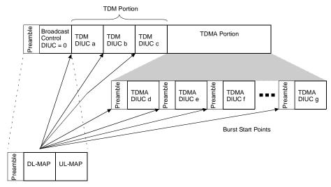
Figure 141—FDD downlink subframe structure
