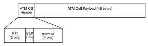
Figure 5—CS PDU format for VC-switched ATM connections
