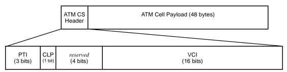
Figure 4—CS PDU format for VP-switched ATM connections
