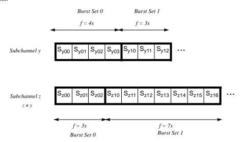
Figure 191—Segment alignment for overlapping burst sets on different subchannels
