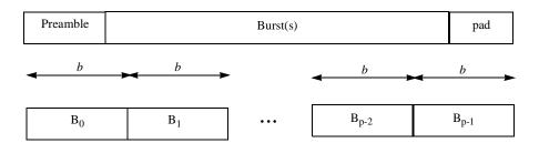
Figure 186—Base frame partitioning and padding
