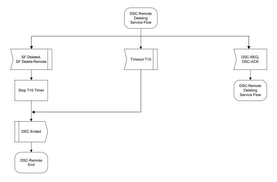
Figure 123—DSC—Remotely Initiated Transaction Deleting Service Flow state flow diagram
