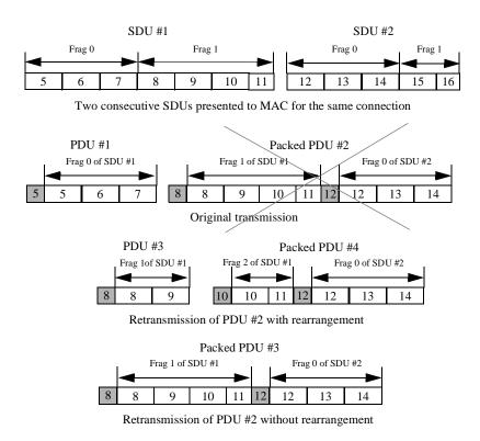
Figure 32—Block usage examples for ARQ with and without rearrangement
