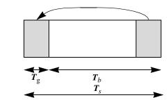
Figure 195—OFDM symbol time structure
