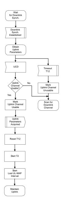
Figure 58—Obtaining uplink parameters
