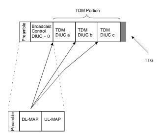
Figure 140—TDD downlink subframe structure
