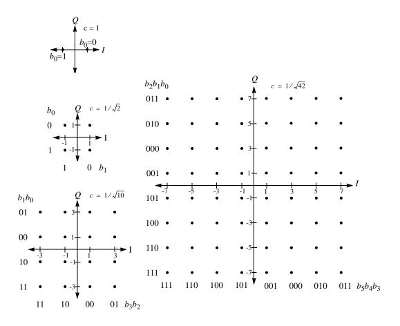
Figure 203—BPSK, QPSK, 16-QAM, and 64-QAM constellations
