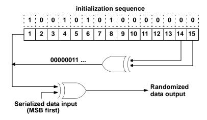
Figure 146—Randomizer logic diagram
