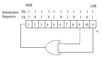
Figure 262—PRBS for pilot modulation
