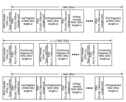
Figure 28—Packing with fragmentation
