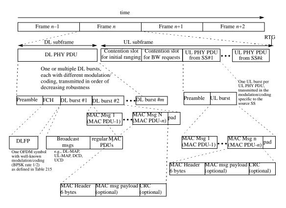
Figure 207—Example of OFDM frame structure with TDD
