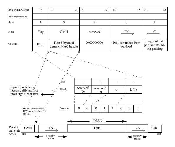
Figure 137—Construction of Ai
