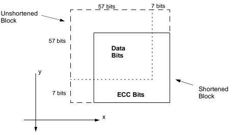
Figure 150—Structure of shortened 2 D block
