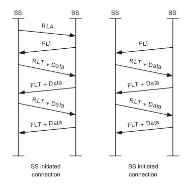
Figure 229—PHY control signal sequence diagrams
