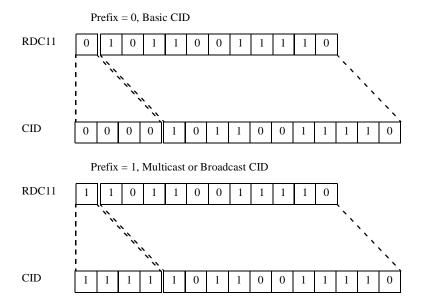
Figure 22—Reduced CID Decoding
