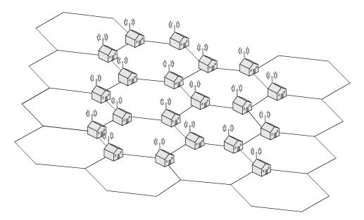
Figure B.1—WirelessHUMAN Mesh deployment model
