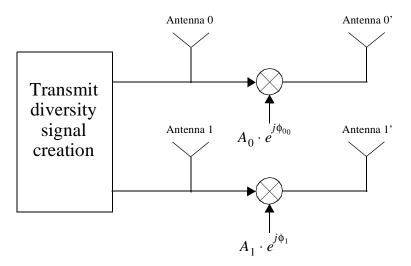
Figure 250—Illustration of Transmit diversity using four antennas
