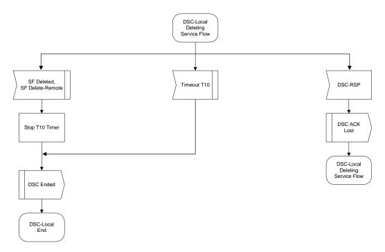
Figure 119—DSC—Locally Initiated Transaction Deleting Service Flow state flow diagram
