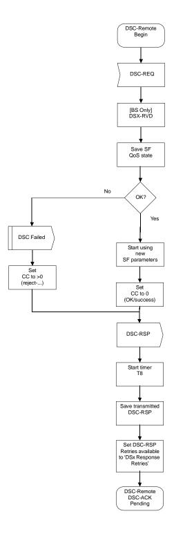
Figure 120—DSC—Remotely Initiated Transaction Begin state flow diagram
