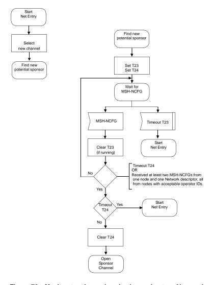
Figure 73—Mesh network synchronization and entry—New node—I
