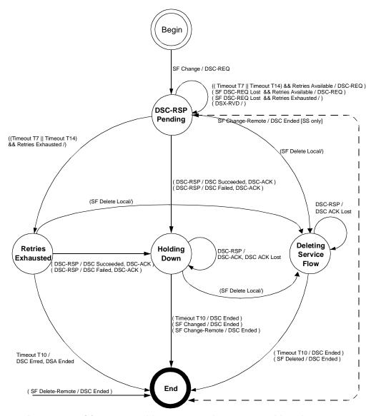
Figure 102—DSC—Locally Initiated Transaction state transition diagram
