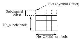
Figure 215—Example of the data region which defines the OFDMA allocation
