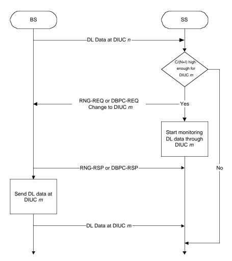
Figure 80—Transition to a less robust burst profile
