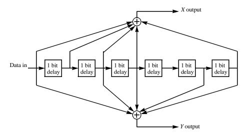
Figure 255—Convolutional encoder of rate 1/2
