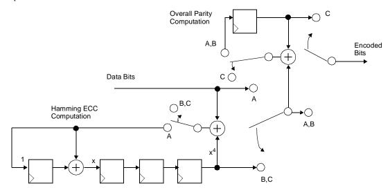
Figure 149—Example encoder for a (16,11) extended Hamming Code
