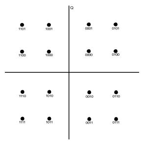
Figure 152—16-QAM constellation (gray-coded)
