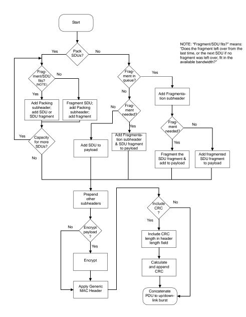
Figure 24—Construction of a MAC PDU
