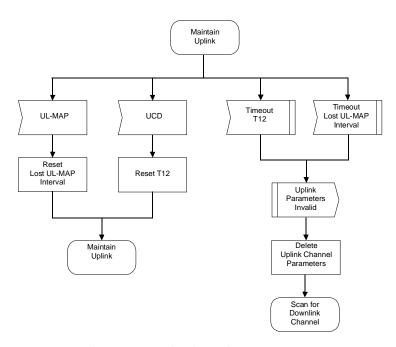
Figure 59—Maintain uplink parameters
