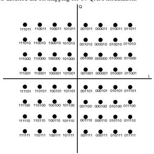
Figure 153—64-QAM constellation (gray-coded)
