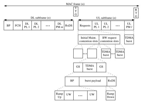
Figure 193—Example of TDD frame format
