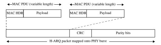
Figure 130—Construction of H-ARQ encoder packet
