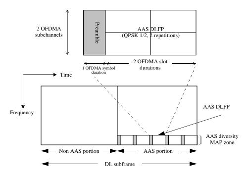
Figure 223—Example of allocation for AAS\_DL\_Scan IE
