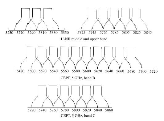
Figure 264—Channelization, 20 MHz
