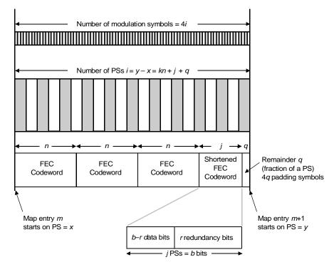
Figure 142—DL-MAP usage with shortened FEC blocks—TDM case
