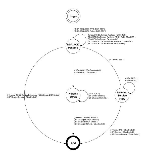
Figure 101—DSA—Remotely Initiated Transaction state transition diagram
