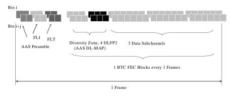
Figure 226—Downlink BW Allocation/Access channel
