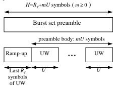
Figure 179—Burst set preamble composition
