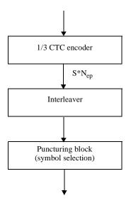
Figure 258—Block diagram of subpacket generation
