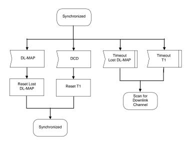
Figure 57—Maintaining downlink synchronization
