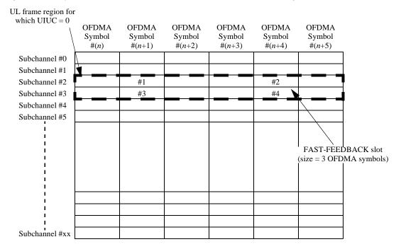
Figure 230—Mapping order of FAST-FEEDBACK messages to the FAST-FEEDBACK region
