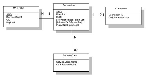
Figure 95—Theory of Operation Object Model
