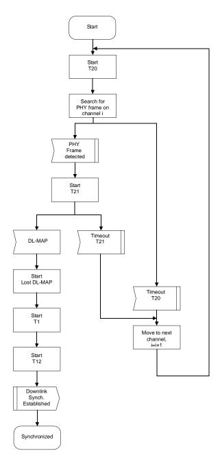
Figure 56—Obtaining downlink synchronization
