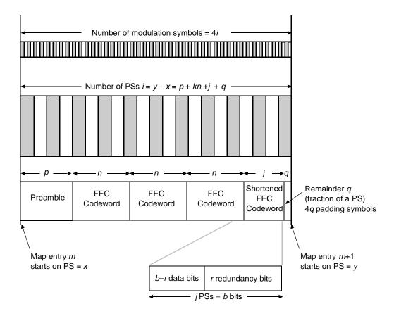
Figure 143—DL-MAP usage with shortened FEC blocks—TDMA case
