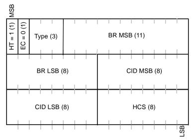
Figure 20—Bandwidth request header format
