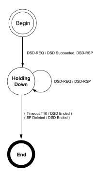
Figure 105—DSD—Remotely Initiated Transaction state transition diagram
