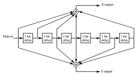
Figure 200—Convolutional encoder of rate 1/2
