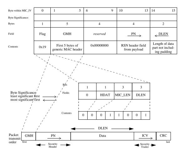
Figure 136—Initial CCM Block B<sub>0</sub>
