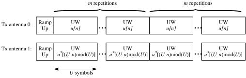
Figure 184—STC burst set preamble
