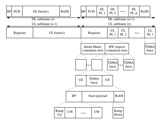
Figure 192—Example of FDD frame format
