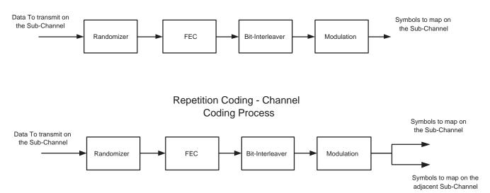
Figure 252—Channel coding process for regular and repetition coding transmission
