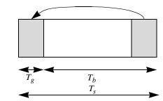
Figure 213—OFDMA symbol time structure
