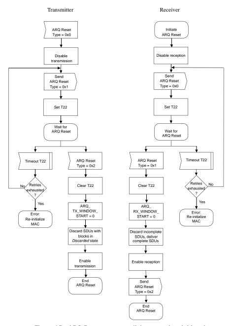
Figure 35—ARQ Reset message dialog—receiver initiated
