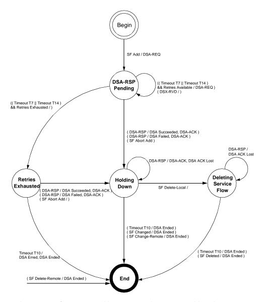
Figure 100—DSA—Locally Initiated Transaction state transition diagram
