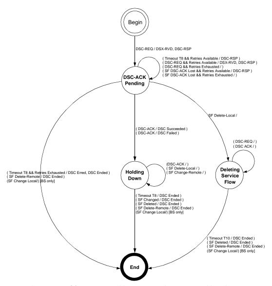
Figure 103—DSC—Remotely Initiated Transaction state transition diagram
