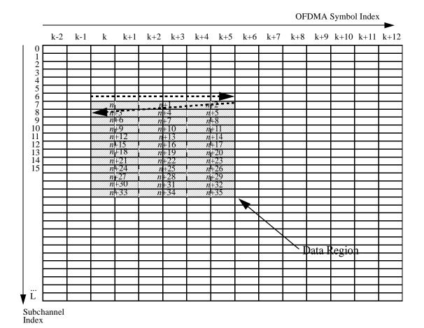
Figure 216—Example of mapping OFDMA slots to subchannels and symbols in the downlink (in PUSC mode)
