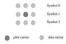
Figure 237—Description of an uplink tile
