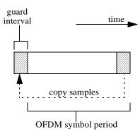
Figure 241—Periodic-ranging or bandwidth-request transmission for OFDMA using one code
