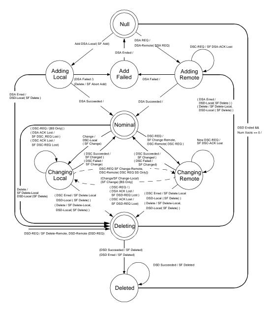
Figure 99—Dynamic Service Flow state transition diagram
