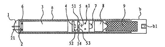
(57) Abstract: An aerosol electronic cigarette includes a battery assembly, an atomizer assembly and a cigarette bottle assembly and also includes a shell (a) which is hollow and integrally formed. Said battery assembly connects with said atomizer assembly and both are located in said shell (a). Said cigarette bottle assembly is located in one end of the shell (a), which is detachable. Said cigarette bottle assembly fits with said atomizer assembly. Said shell (a) has through-air-inlets (a1).
