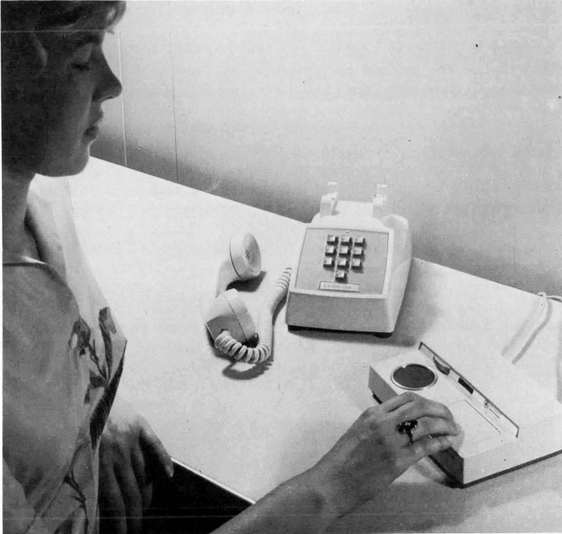
Figure 2-9. COM-CODE set for the handicapped. When connected to conventional telephones, this device allows a deaf person to receive messages via flashes of light or vibrations. The circular vibrating pad is shown on the left of the device, the sending key, which is used like a telegraph key, on the right. Light flashes come from a recess (the black rectangle) to the left of the bell symbol.
