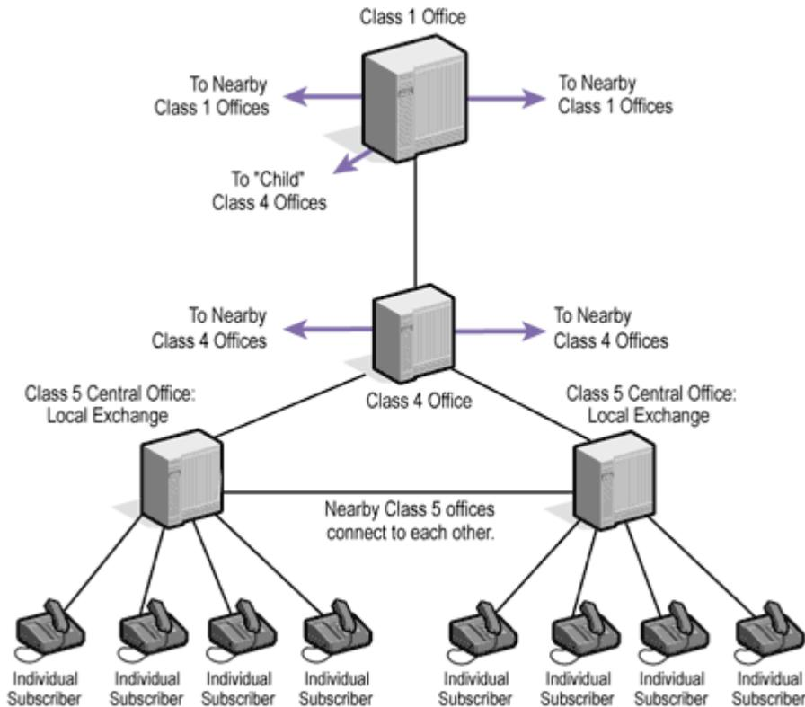
44. The PSTN switch hierarchy does not mandate physical separation. Switches from one or more adjacent classes (specifically edge and tandem) can be located together in the same physical facility. A combined class 4/class 5 switch is often called a “hybrid” switch.
