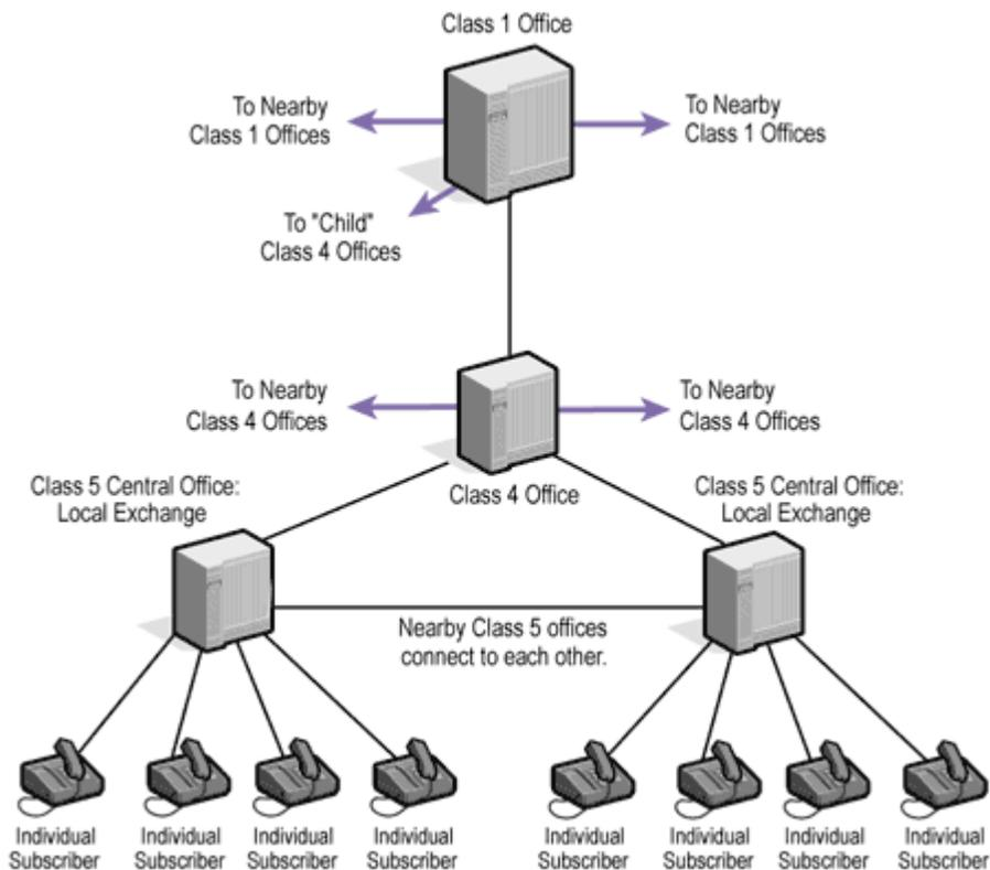
42. The PSTN switch hierarchy does not mandate physical separation. Switches from one or more adjacent classes (specifically edge and tandem) can be located together in the same physical facility. A combined class 4/class 5 switch is often called a “hybrid” switch.
