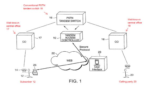
Annotated Figure 1 illustrates tandem access controller 10 connected to conventional Public Service Telephone Network (PSTN) tandem switch 16. *Id.* at 4:60–64. According to the '298 patent, "[d]etails of the operation of the existing phone network," including directing of phone calls by "existing" PSTN tandem switch 16 to central offices 17, 18 are further described in a publication incorporated by reference, as well as "numerous books describing the PSTN." *Id.* at 4:60–5:4.
