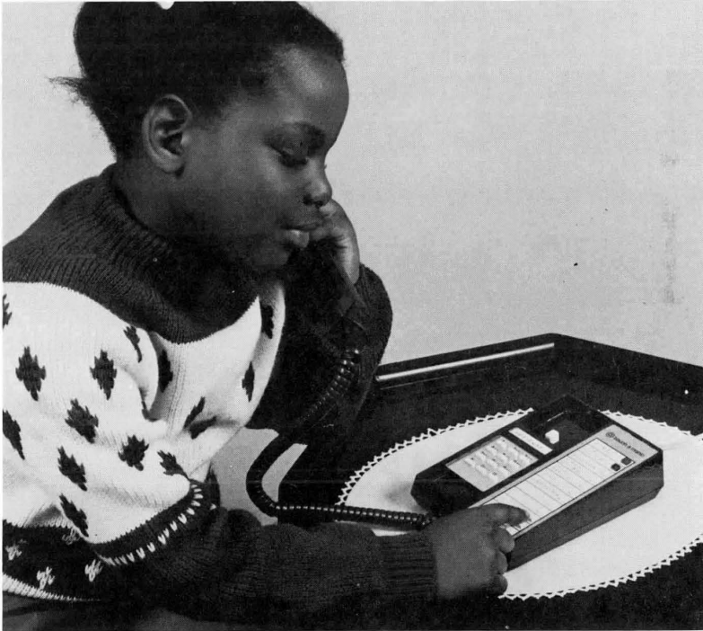
Figure 2-4. TOUCH-A-MATIC S series telephone, the Bell System's first microprocessor-based telephone for the home. Important or frequently called numbers can be dialed at the touch of a button. Red and green buttons at the top of the panel identify emergency numbers.
