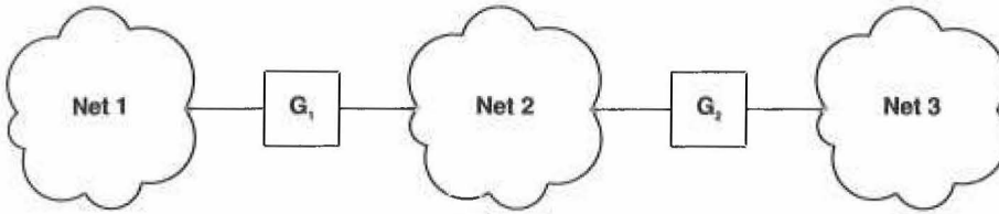
Figure 3.2 Three networks interconnected by two gateways.
