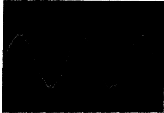
Fig. 5. Waveform of a 101-stage enhancement/depletion ring oscillator consisting of 0.2- \mu\text{m} MOSFET's with 75-nm gate oxide at a power supply voltage of 3 V. The output signal is 75 mV peak to peak (20 mV/div).
