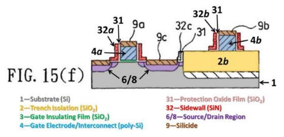
The figure above depicts a device including isolation 2b, which is the result of forming a trench in silicon substrate 1 and filling it with insulating
