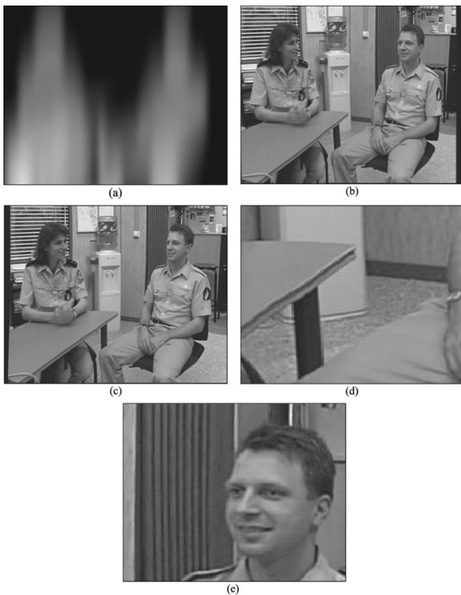
Fig. 7. Virtual images generated using asymmetric smoothing of the depth map with \sigma_\mu = 10 and \sigma_v = 90 . (a) Depth map after asymmetric smoothing; (b) virtual left-eye image; (c) virtual right-eye image; (d) and (e) enlarged segments from the image shown in (b). Note vertical lines are now straight compared to Fig. 5(e).
