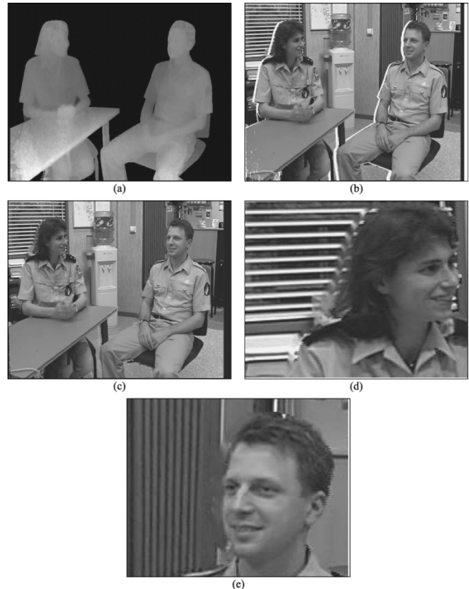
Fig. 4. Virtual left-eye image generated without smoothing of the depth map. (a) Depth map without smoothing; (b) image after 3D image warping. White areas represent newly exposed areas; (c) image after hole-filling ; (d) and (e) artifacts clearly seen in enlarged segments of the image from (c).
