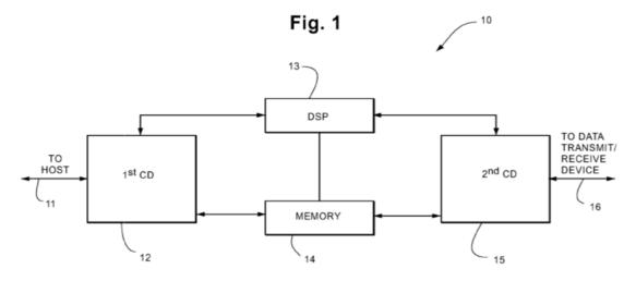
As shown in Figure 1 above, interface device 10 connects to a host device via host line 11, and to a data transmit/receive device via output line 16. *Id.* at 4:59–5:10. Interface device 10 includes first connecting device 12, second connecting device 15, digital signal processor 13, and memory means 14. *Id.* In a preferred embodiment, the interface device is attached to a host device via a multi-purpose interface—e.g., a small computer systems
