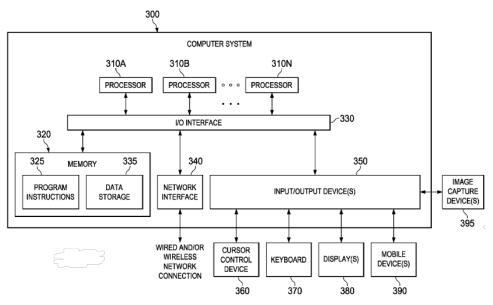
Figure 3 depicts a schematic diagram of computer system 300 that includes processors 310, system memory 320, program instructions 325, and I/O interface 330 that connects to input/output devices 350. *Id.* at 6:39–8:15.
