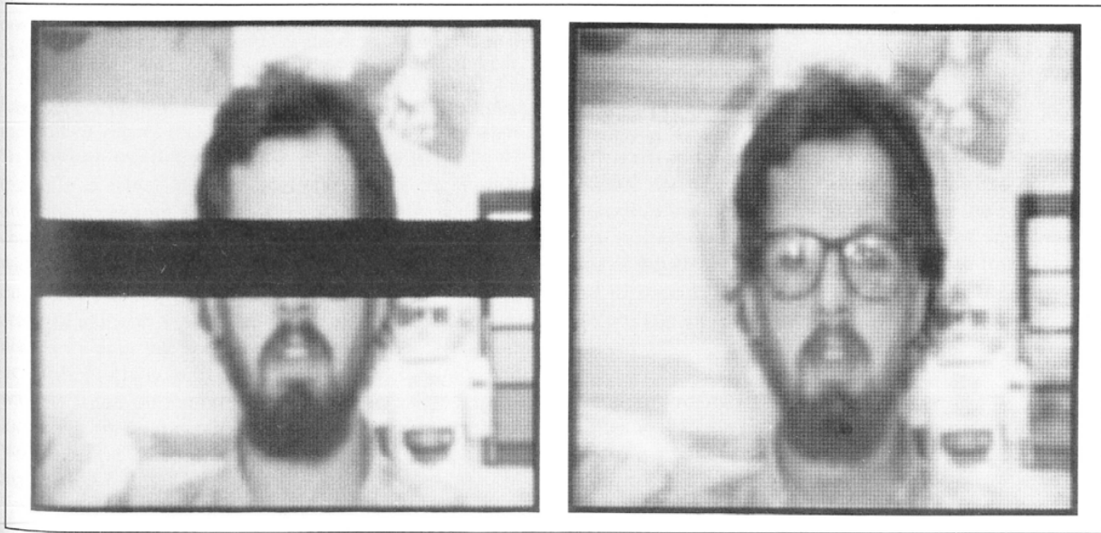
Figure 13. (a) Partially occluded face image and (b) its reconstruction using the eigenfaces.
