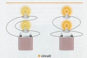
Bulbs in a series circuit (left) give off dim light since they each consume a portion of the power coming through a single circuit connected to the battery. In a parallel circuit (right) bulbs shine brightly since each is directly connected in its own circuit to the power source.
