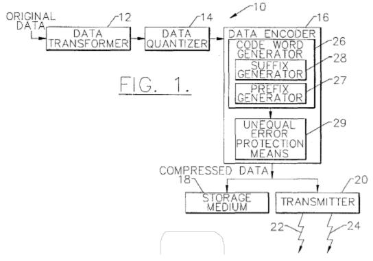
Figure 1 above shows a block diagram of error resilient data compression apparatus 10, including error resilient data encoder 16. *Id.* at 8:48–51. Original data is initially transformed by data transformer 12. *Id.* at 9:30–32. The original data can be transformed based upon one of a number of predetermined functions, such as a cosine function, a complex
