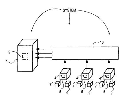
Figure 1 is a block diagram showing the components and data flow of a computerized human communication arbitrating and distributing system. *Id.* at 4:60–64. The system includes a controller computer (shown as 1 in Figure 1 but described as 3 in the written description) in communication with several participator computers 5 (e.g., IBM-compatible personal
