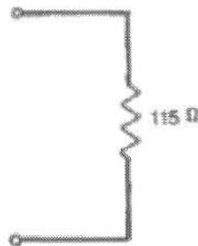
Fig 12-17 Simulated Light Load
