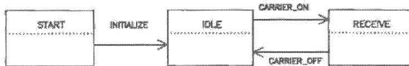
Fig B2 Receive Component State Diagram
