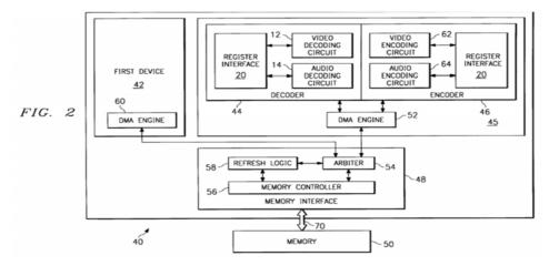
As shown in Figure 2, electronic system 40 includes first device 42, decoder 44, encoder 46, memory interface 48, and memory 50. Ex. 1001,
