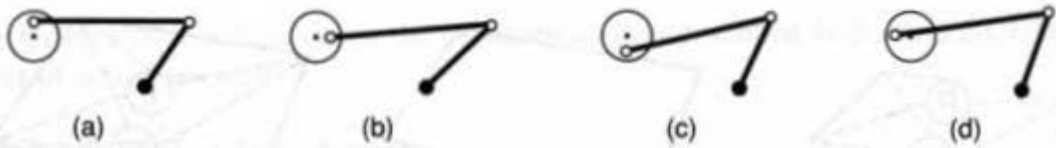
Fig. 21.7 The linkage in (a) is moved by rotating the drive wheel. The constraints generate the motions shown in (b), (c), and (d).
