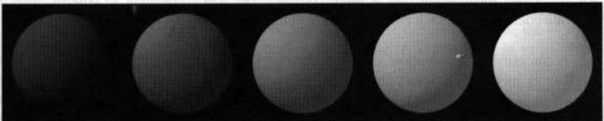
Fig. 16.4 Spheres shaded using ambient and diffuse reflection (Eq. 16.5). For all spheres, I_a = I_p = 1.0 , k_d = 0.4 . From left to right, k_a = 0.0, 0.15, 0.30, 0.45, 0.60 . (By David Kurlander, Columbia University.)
