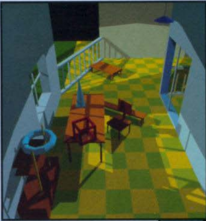
Plate III.6 Room with shadows generated by object-precision shadow-volume BSP tree algorithm of Section 16.4.3. (a) Scene with two point light sources. (b) Same scene with black lines indicating polygon fragmentation. Dark gray fragments are lit by no lights, light gray fragments are lit by one light, and non-gray fragments are lit by both lights. (Courtesy of Norman Chin, Columbia University.)
