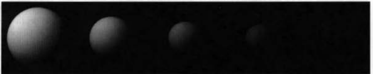
Fig. 16.7 Spheres shaded using depth cueing (Eqs. 16.5, 16.11, and 16.12). Distance from light is constant. For all spheres, I_s = I_o = 1.0 , k_s = 0.1 , k_d = 0.9 , z_f = 1.0 , z_b = 0.0 , s_f = 1.0 , s_b = 0.1 , radius = 0.09. From left to right, z at front of sphere is 1.0, 0.77, 0.55, 0.32, 0.09. (By David Kurlander, Columbia University.)
