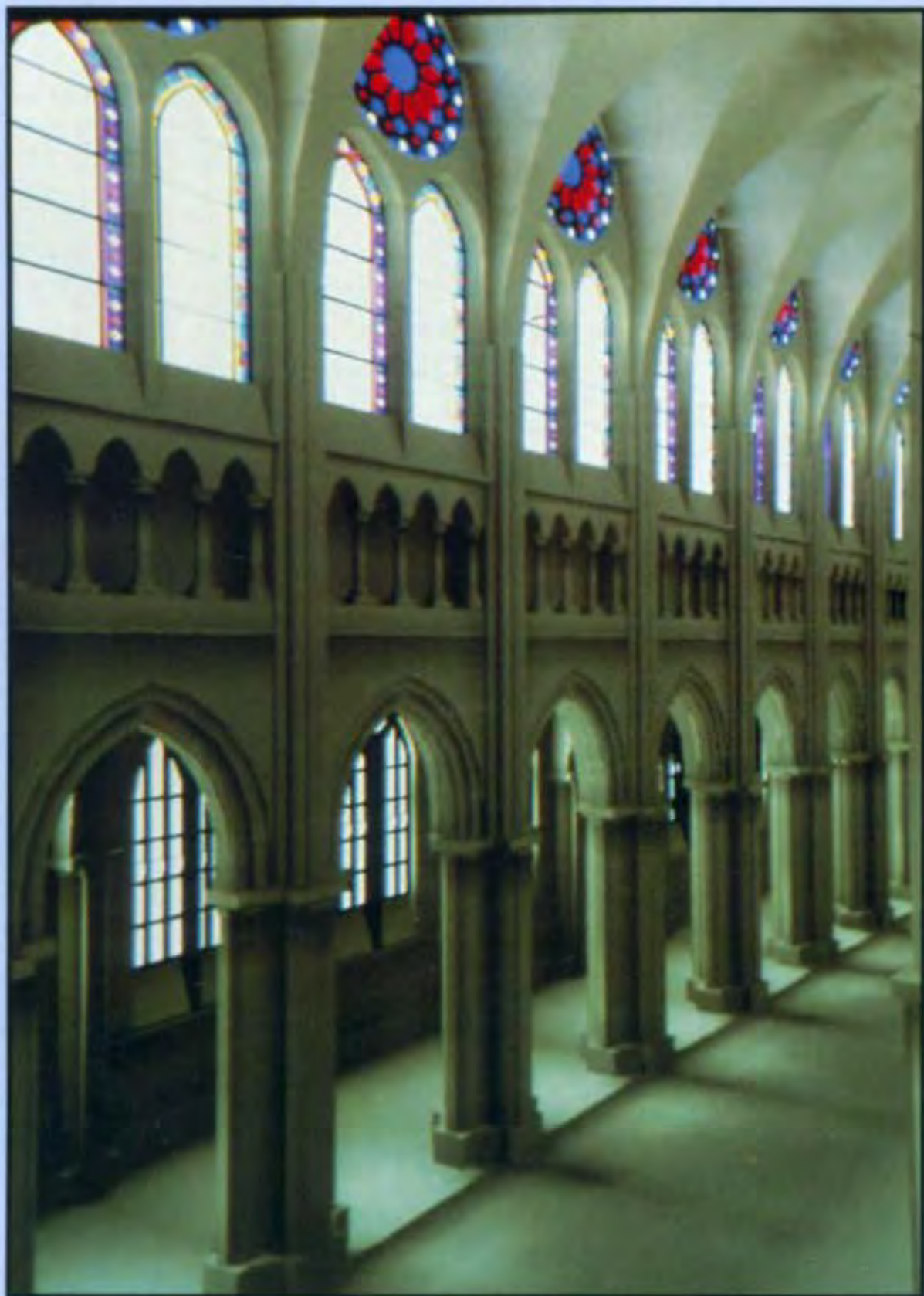
Plate III.24 Nave of Chartres cathedral rendered with progressive-refinement radiosity algorithm, using ray tracing to compute form factors (Section 16.13.5). Two bays, containing 9916 polygons, were processed and copied three more times. Sixty iterations took 59 minutes on HP 9000 Model 835 TurboSRX. (By John Wallace and John Lin, using Hewlett-Packard's Starbase Radiosity and Ray Tracing software. © 1989, Hewlett-Packard Co.)
