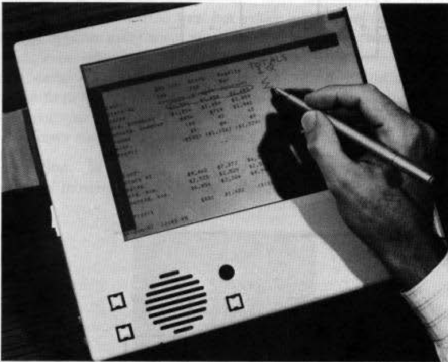
Fig. 8.19 An IBM experimental display and transparent data tablet. A spreadsheet application is executing. The user has just circled three numbers, and has indicated that their sum is to be entered in the cell containing the sigma. A new column heading has also been printed. The system recognizes the gestures and characters, and enters appropriate commands to the spreadsheet application. (Courtesy IBM T. J. Watson Research Laboratories.)
