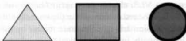
Fig. 9.22 A triply redundant code using line thickness, geometric shape, and interior fill pattern. Any one of the three codes is sufficient to distinguish between the three code values.
