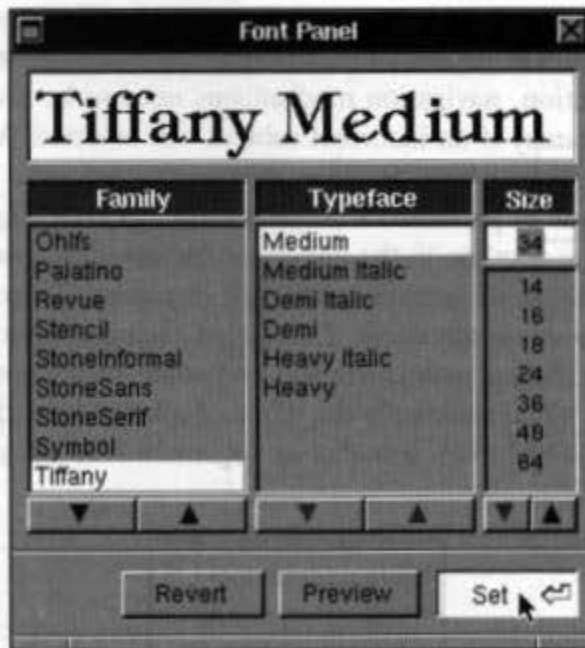
Fig. 8.11 A hierarchical-selection menu. The leftmost column represents the top level; the children of the selected item in this column are shown in the next column; and so on. If there is no selected item, then the columns to the right are blank. (Courtesy of NeXT, Inc. © 1989 NeXT, Inc.)
