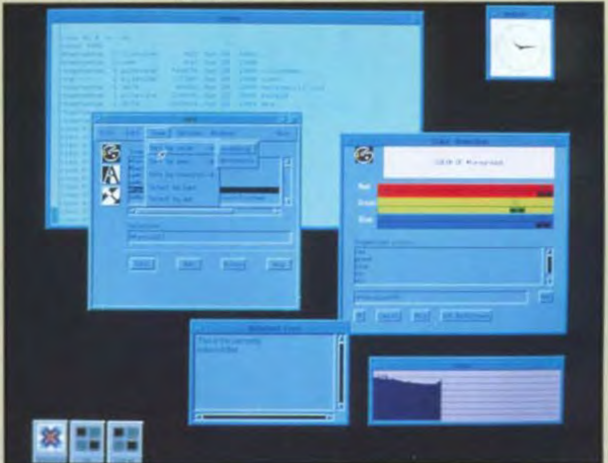
Plate I.27 The OSF/Motif user interface. The color slider bars are used to define colors for use in windows. Notice the use of shading on the edges of buttons, menus, and so forth, to create a 3D effect. (Courtesy of Open Software Foundation.)
