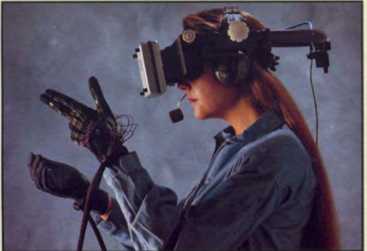
Plate I.16 A user wearing a head-mounted stereo display, DataGloves, and microphone for issuing commands. These devices are used to create a virtual reality for the user, by changing the stereo display presentation as the head is moved, with the DataGloves used to manipulate computer-generated objects. (Courtesy of Michael McGreevy and Scott Fisher, NASA Ames Research Center, Moffett Field, CA.)
