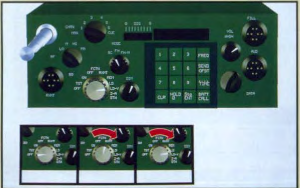
Plate I.25 Picture of a radio generated by IBIS to satisfy input communicative goals to show location of function dial and its change of state. IBIS determines the objects to include, rendering style, viewing and lighting specs, and picture composition. (Courtesy of Dorée Duncan Seligmann and Steven Feiner, Columbia University.)
