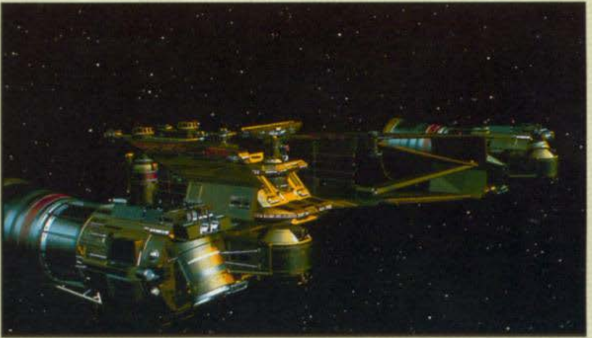
Plate I.13 Command ship from The Last Starfighter . The texture-mapped ship has 450,000 polygons. (Copyright © 1984 Digital Productions. Courtesy of G. Demos.)
