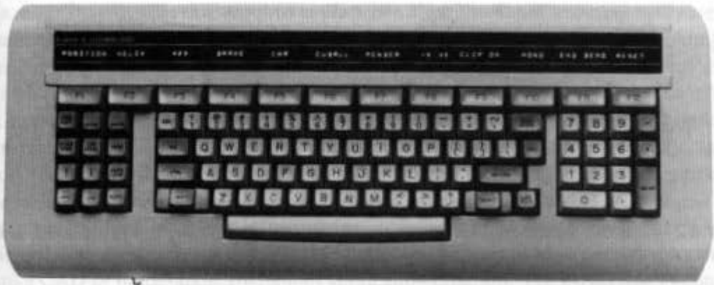
Fig. 4.41 Function keys with light-emitting diode (LED) labels, integrated with a keyboard unit. (Courtesy of Evans and Sutherland Computer Corporation.)
