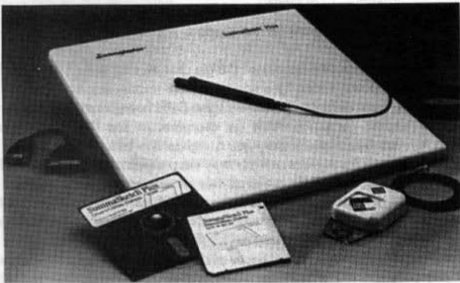
Fig. 4.34 A data tablet with both a stylus and a puck. The stylus has a pressure-sensitive switch in the tip, which closes when the stylus is pressed. The puck has several pushbuttons for command entry, and a cross-hair cursor for accuracy in digitizing drawings that are placed on the tablet. (Courtesy of Summagraphics Corporation.)
