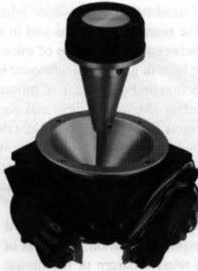
Fig. 4.38 A joystick with a third degree of freedom. The joystick can be twisted clockwise and counterclockwise. (Courtesy of Measurement Systems, Inc.)
