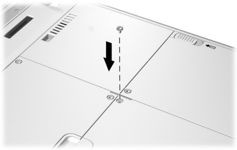
Inserting a battery pack security screw
