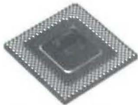
Pin grid array. The pin grid array on the back of a Pentium chip.
