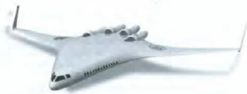
Fig. 2 A 3-D rendering of a candidate Silent Aircraft airframe and propulsion system, taken from [11]
