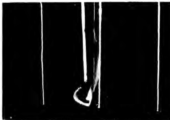
FIGURE 291.—Displacement of passage vortex by tip-clearance vortex (ref. 318).
