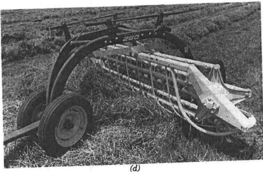
Figure 8.33—A side delivery rake with oblique reel-head (Courtesy of Ford-New Holland, Inc.).
