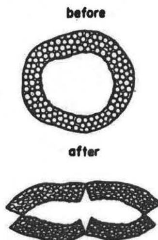
Figure 8.13—Cross-section of a stem (a) before and (b) after compression (Reprinted from Mechanics of Cutting Plant Materials , Persson, 1987).
