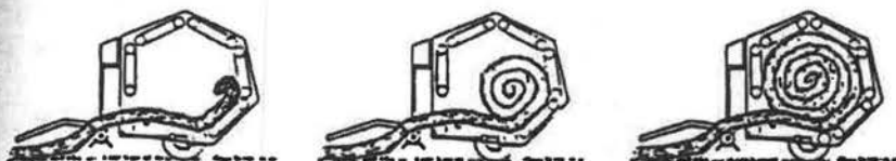
Figure 8.42—A round baler with fixed geometry (Courtesy of Prairie Agricultural Machinery Institute, Canada).
