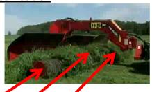
First, second, and third pickup assemblies aligned side by side; providing an unobstructed continuous line of material pickup
