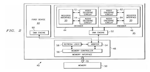
As shown in Figure 2, electronic system 40 includes first device 42, decoder 44, encoder 46, memory interface 48, and memory 50. Ex. 1001,
