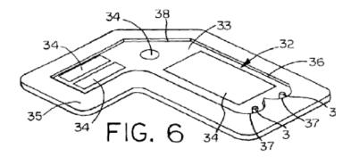
Fig. 6 is a schematic view of a light emitting panel assembly.
