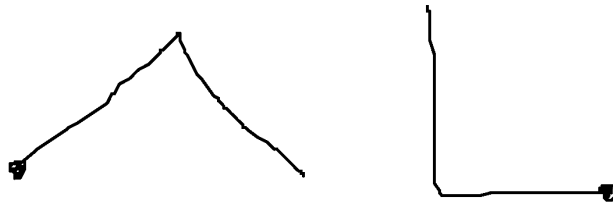
Figure 6.7: Two marking menu marks that are augmented by a “dot” to distinguish them from other types of marks in an interface.
