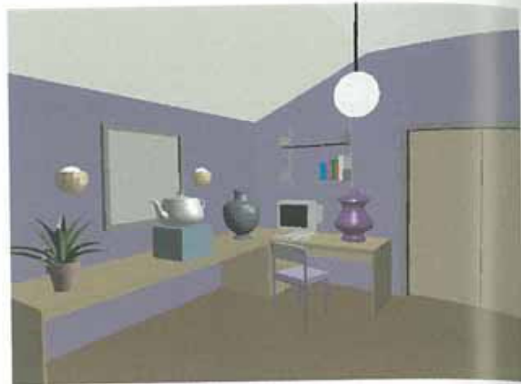
Figure 18.2 The same scene using flat shading. Flat shading shows the polygonal nature of the surfaces due to discontinuities in intensity.
