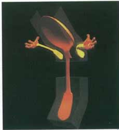
Figure 3.42 FFD applied to a polygon mesh object. (a) Wireframe of the object. (b) The object rendered with the trivariate patch grid shown as semi-transparent grey boxes. (c) Moving the control points in the patch causes the object model to deform in an appropriate manner.
