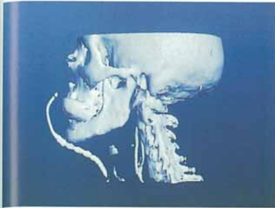
Figure 13.10 The marching cubes algorithm applied to X-ray CT data. (Courtesy of Klaus de Geuss.)
