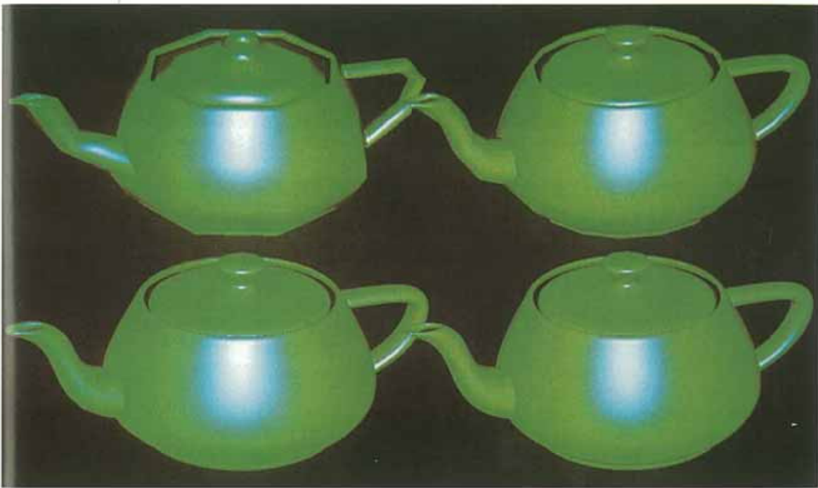
Figure 4.9 Parametric patch rendering at different levels of uniform subdivision (128, 512, 2048 and 8192 polygons). (Courtesy of Steve Maddock.)
