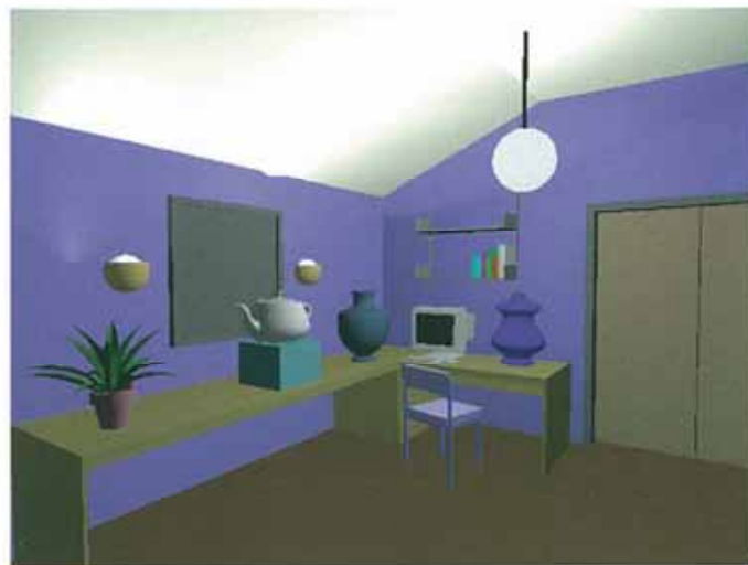
Figure 18.5 The same scene using Phong shading. A glaring defect in Phong interpolation is demonstrated in this figure. Here the reflected light from the wall light and the image of the light have become separated due to the nature of the interpolation.
