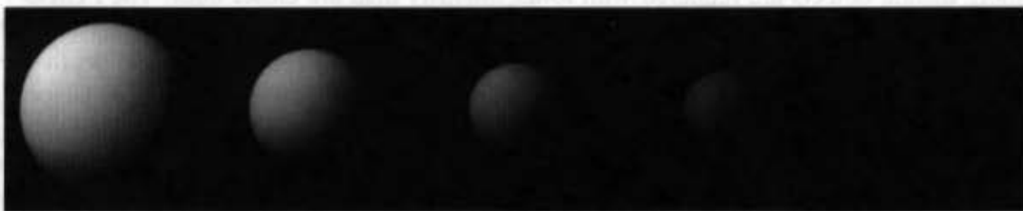
Fig. 16.7 Spheres shaded using depth cueing (Eqs. 16.5, 16.11, and 16.12). Distance from light is constant. For all spheres, I_s = I_p = 1.0 , k_s = 0.1 , k_d = 0.9 , z_f = 1.0 , z_b = 0.0 , s_f = 1.0 , s_b = 0.1 , radius = 0.09. From left to right, z at front of sphere is 1.0, 0.77, 0.55, 0.32, 0.09. (By David Kurlander, Columbia University.)
