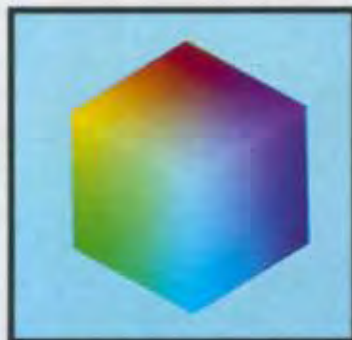
Plate II.5 An interior subcube of the RGB color space. The gray vertex is at (0.5, 0.5, 0.5) Hence the subcube is half the height, width, and depth of the entire space shown in Color Plate II.4. (Courtesy of David Small, Visible Language Workshop, MIT Media Lab, Cambridge, MA 02139. © MIT, 1989.)
