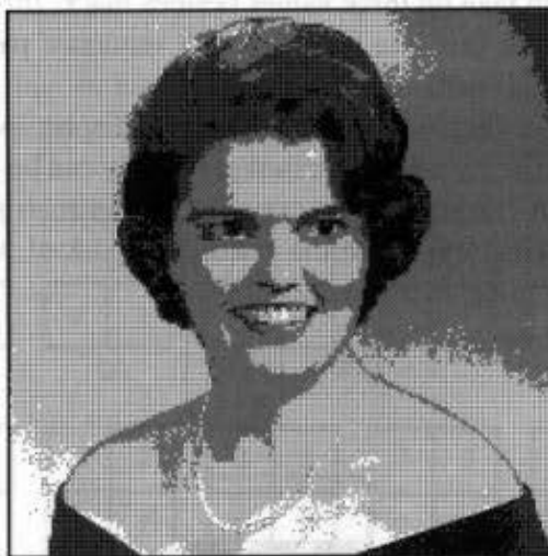
Fig. 13.9 A continuous-tone photograph, digitized to a resolution of 351 \times 351 and displayed using the 2 \times 2 patterns of Fig. 13.8. (Courtesy of Alan Paeth, University of Waterloo Computer Graphics Lab.)
