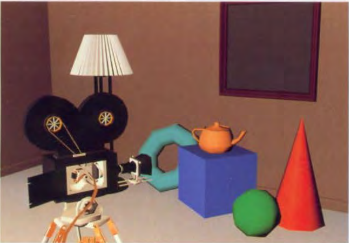
Plate II.30 Shutterbug . Gouraud shaded polygons with diffuse reflection (Sections 14.4.3 and 16.2.4). (Copyright © 1990, Pixar. Rendered by Thomas Williams and H.B. Siegel using Pixar's PhotoRealistic RenderMan™ software.)
