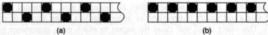
Fig. 13.41 Results obtained by using intensity level 1 from Fig. 13.8 in two ways: (a) with alternation (intensified pixels are on both scan lines), and (b) without alternation (all intensified pixels are on the same scan line).
