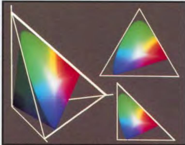
Plate II.1 Several views of the X + Y + Z = 1 plane of CIE space. Left: the plane embedded in CIE space. Top right: a view perpendicular to the plane. Bottom right: the projection onto the (X, Y) plane (that is, the Z = 0 plane), which is the chromaticity diagram. (Courtesy of Barbara Meier, Brown University.)
