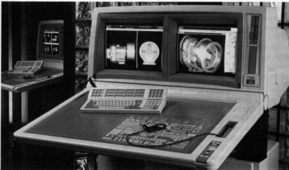
Fig. 8.12 A dual-display workstation. The two displays can be used to show the overview of a drawing on one and detail on the other, or to show the drawing on one and menus on the other. (Courtesy of Intergraph Corporation, Huntsville, Al.)
