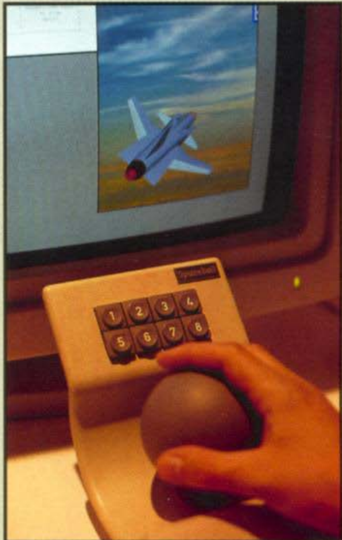
Plate I.14 A spaceball six-degree of freedom positioning device. (Courtesy of Spatial Systems, Inc.)
