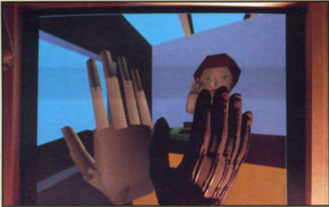
Plate I.15 A DataGlove (right) and computer image of the glove. The DataGlove measures finger movements and hand orientation and position. The computer image of the hand tracks the changes. (Courtesy of Jaron Lanier, VPL.)
