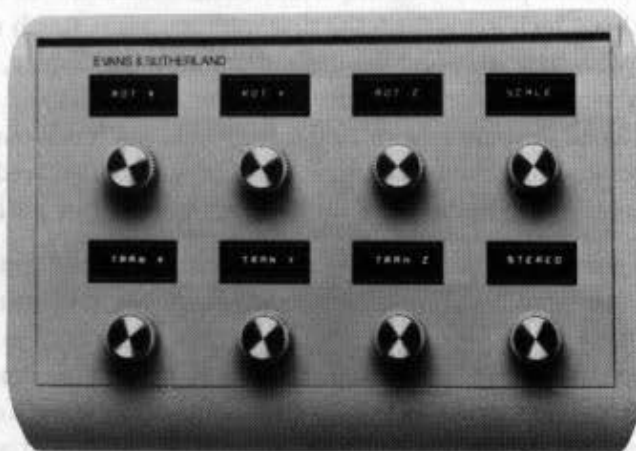
Fig. 4.40 A bank of eight rotary potentiometers. The readouts on the light-emitting diodes (LED) above each dial can be used to label each dial, or to give the current setting. (Courtesy of Evans and Sutherland Computer Corporation.)
