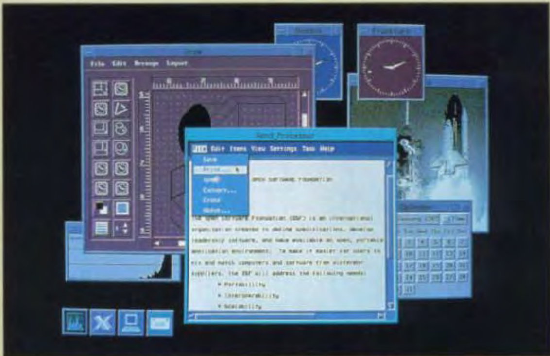
Plate I.26 The OSF/Motif user interface. In this image, different shades of blue are used to distinguish visual elements. (Courtesy of Open Software Foundation.)
