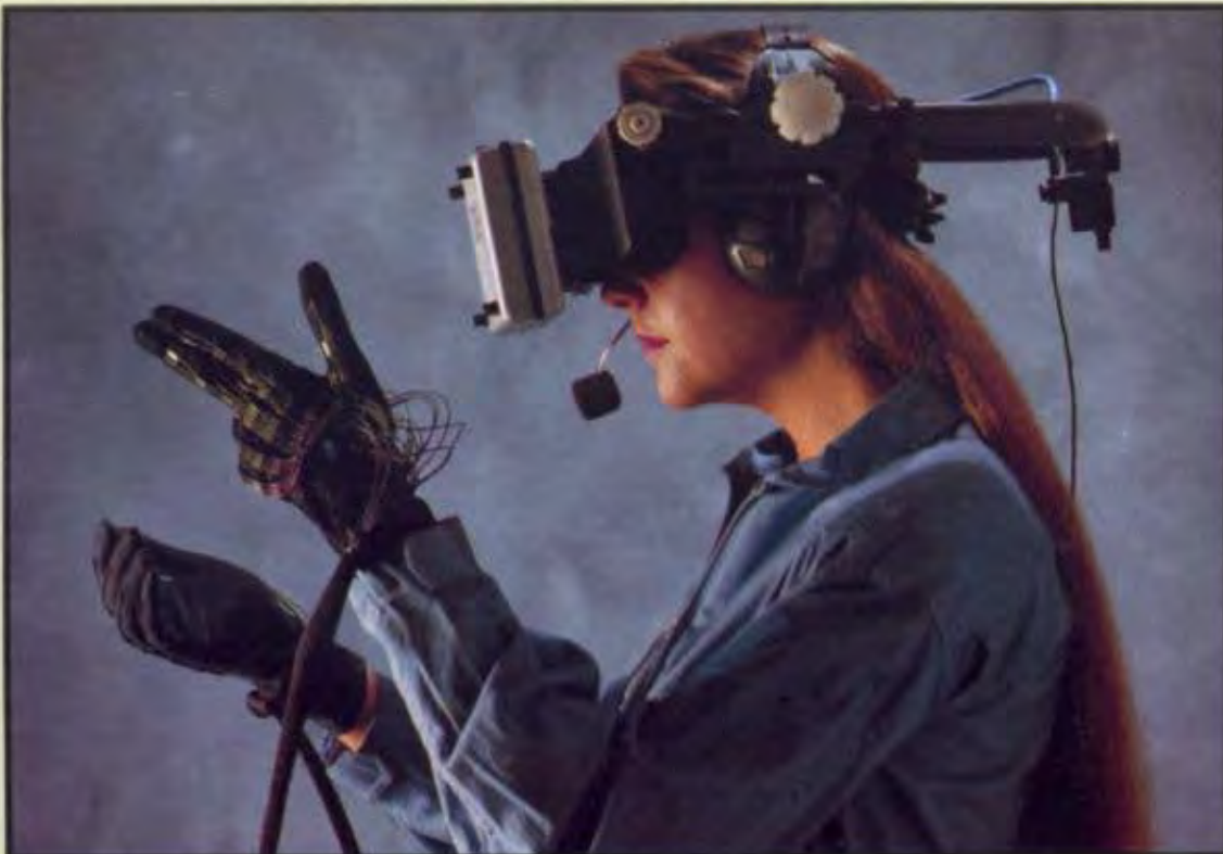
Plate I.16 A user wearing a head-mounted stereo display, DataGloves, and microphone for issuing commands. These devices are used to create a virtual reality for the user, by changing the stereo display presentation as the head is moved, with the DataGloves used to manipulate computer-generated objects. (Courtesy of Michael McGreevy and Scott Fisher, NASA Ames Research Center, Moffett Field, CA.)
