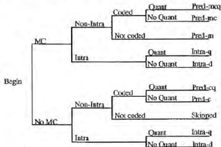
Figure D.32 - Selection of macroblock types in P-pictures
