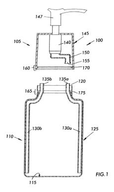
Figure 1 depicts a cross-sectional view of an exemplary dispenser assembly 100. *Id.* at 2:30–31. Dispenser assembly 100 includes container 110, in which any number of passageways 130a, 130b may be mounted, and also includes pump cap 105, in which pump passageway 150 is provided. *Id.* at 2:50–51, 2:63–65, 3:10–14, 3:36–44.
